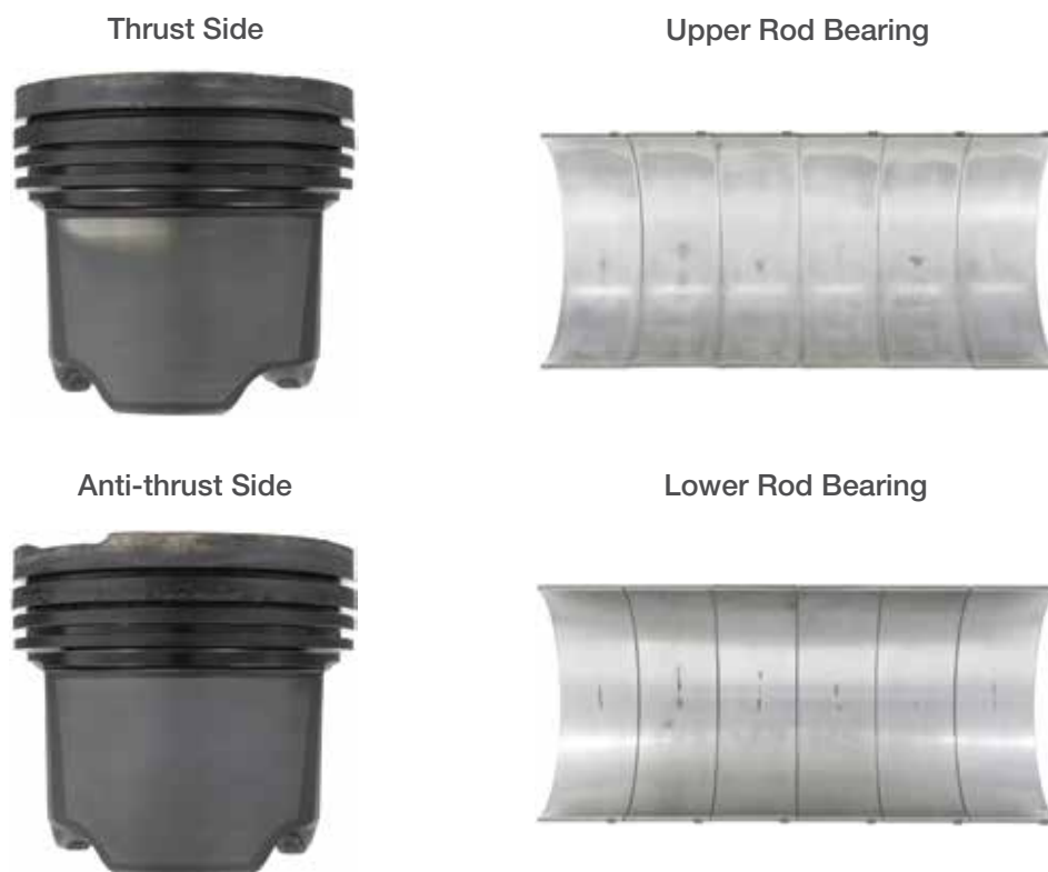
Figure 4. SAE 5W-20 2.6 HTHS parts protection proof of performance field testing. Over 550,000 miles accumulated on Freightliner DD15 with no issues, clean pistons (rear of engine piston #6) with minimal wear on rod bearings.
