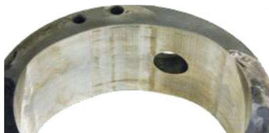
Cam Ring from Parker T6H20C Pump after Wet Phase with HiTEC®523 in Group I Basestocks
