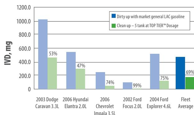
Excellent performance in PFI engines as shown by the 69% fleet average clean-up of intake valve deposits.
