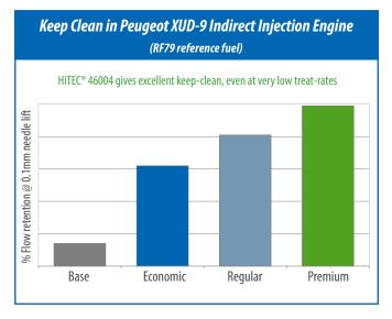
HiTEC® 46004 keeps deposits from forming that typically build up when using untreated base fuel.
